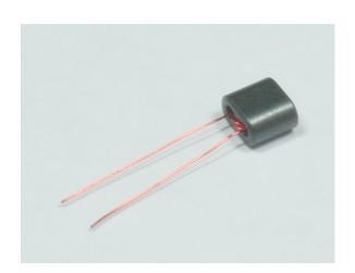
On the opposite end, repeat the process of winding either 4 or 5 turns on the core, keeping the turns tight and neat. If winding 5 turns on the core, mark that end (on the core) so it can be installed correctly.
