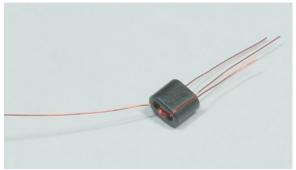
Trim all of the wires to approximately 1 inch, remove the insulation, then tin each lead as shown. T1 is now complete and ready to install into the PCB.
