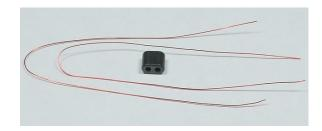
Bend a wire back on itself about 1.25 inches and insert into the core from one end. Snug this first turn up tightly, but not to the point of breaking the wire.
