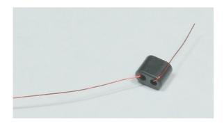
Wind on an additional 3 turns, keeping the turns tight and organized on the core. A turn is counted when the wire goes through a core hole and back through to the opposite side. When 4 turns have been wound on the core, the opposite end from where the wires exit will show 4 turns.
