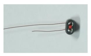
When 4 turns have been wound on, trim off the excess wire leaving about 1 inch long leads.
